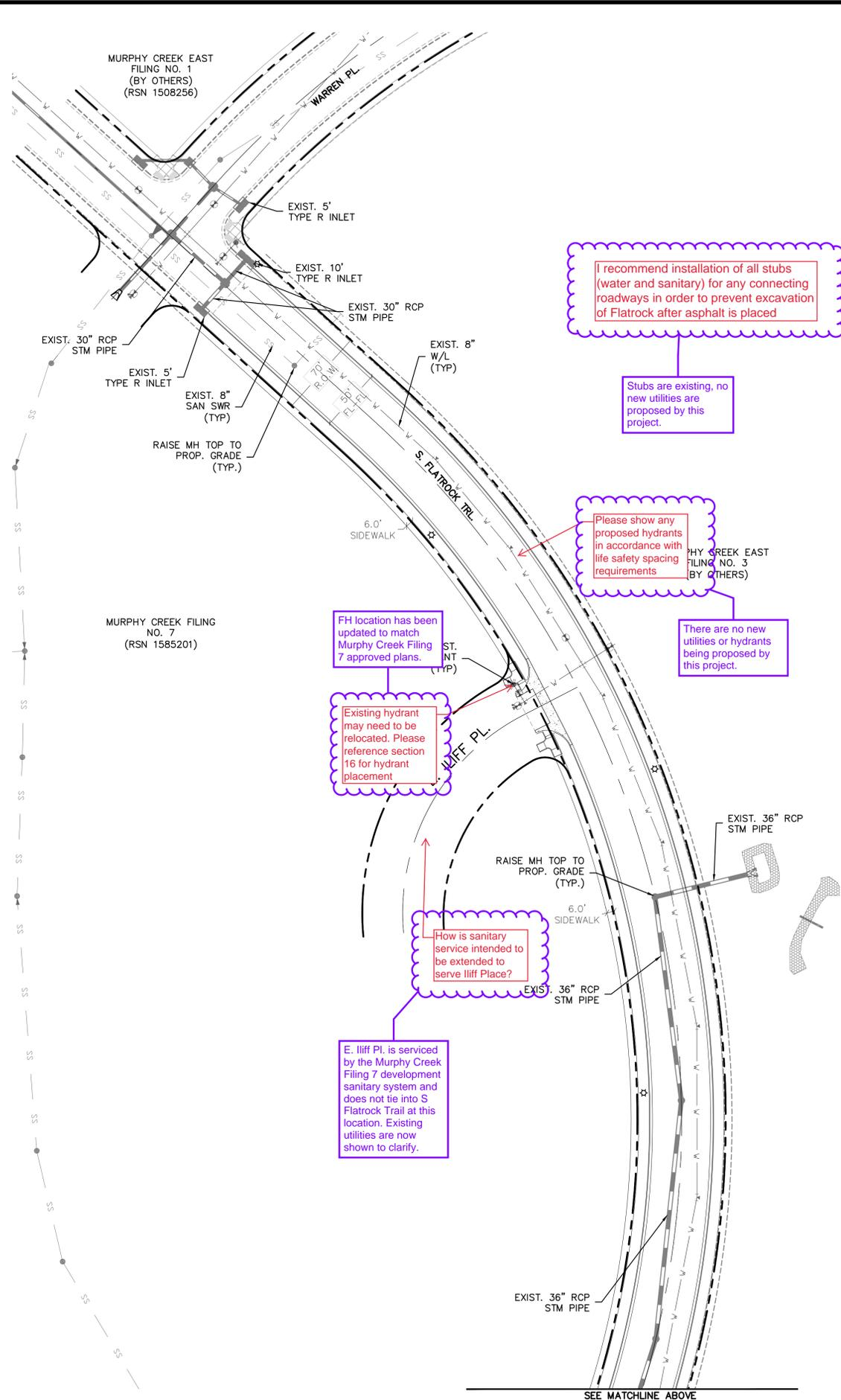
I recommend installation of all stubs (water and sanitary) for any connecting roadways in order to prevent excavation of Flatrock after asphalt is placed
