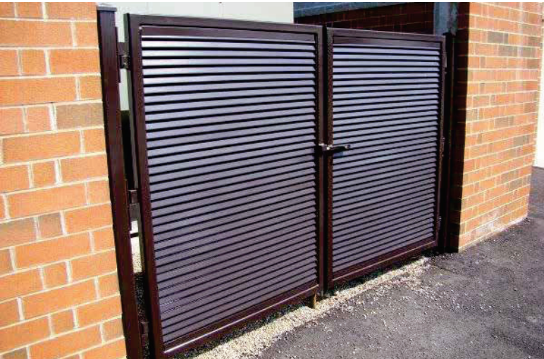
Trash Enclosure with metal panel gates and masonry surround
