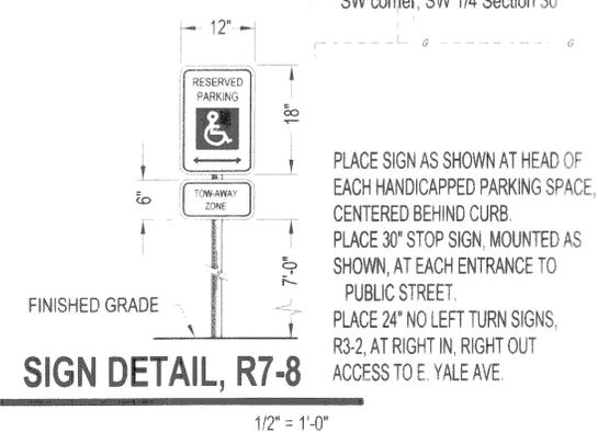
ALL SIGNS SHALL CONFORM TO THE MANUAL ON UNIFORM TRAFFIC CONTROL DEVICES.
