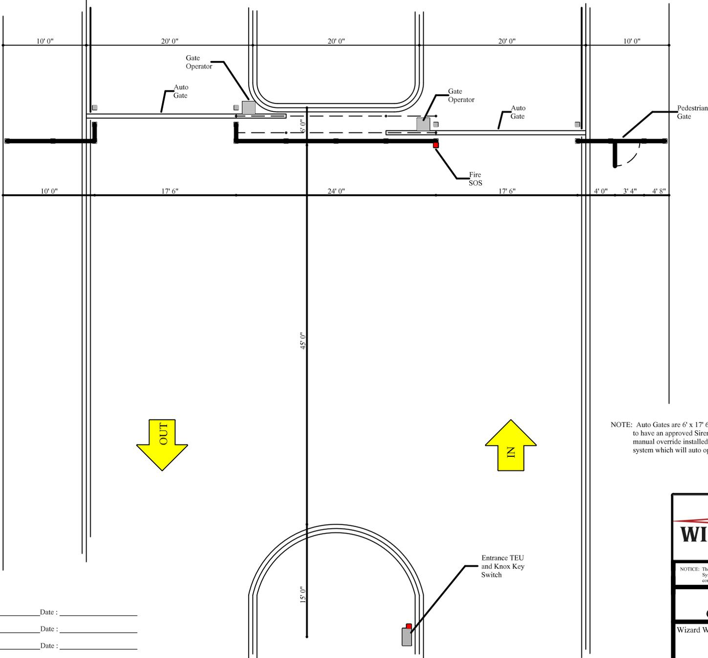
NOTE: Auto Gates are 6' x 17' 6" cantilever Slide Gates. These gates are to have an approved Siren Operated System, KNOX keyswitch, and manual override installed. In addition they will have a battery backup system which will auto open the gates in the event of a power outage.
