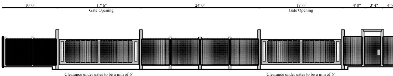
NOTE: Auto Gates are 6' x 17' 6" cantilever Slide Gates. These gates are to have an approved Siren Operated System, KNOX keyswitch, and manual override installed. In addition they will have a battery backup system which will auto open the gates in the event of a power outage.
