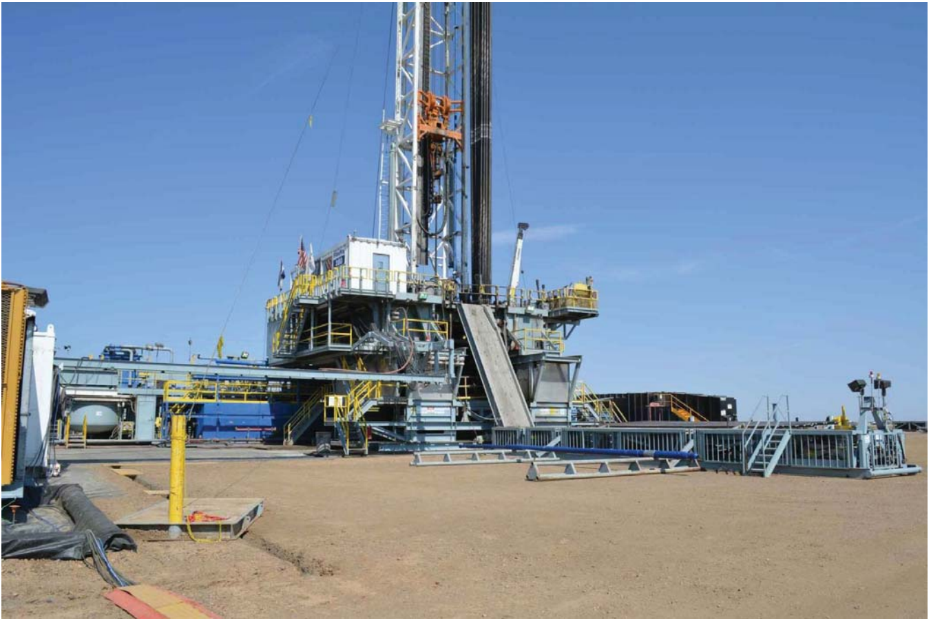
AURORA COLORADO OIL & GAS OPERATIONS DRILLING RIG WITH AUTOMATIC PIPE HANDLING
