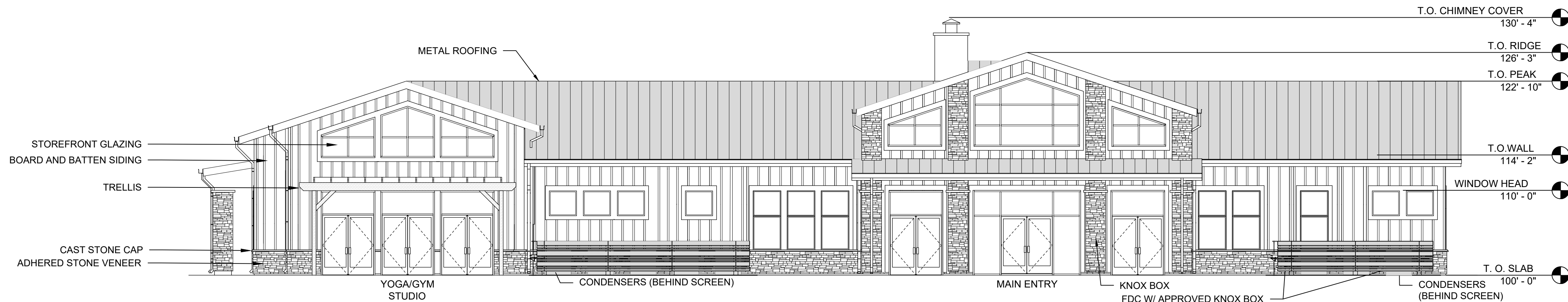
A EAST ELEVATION (FRONT ENTRY) SCALE: 1/8"=1'-0"
