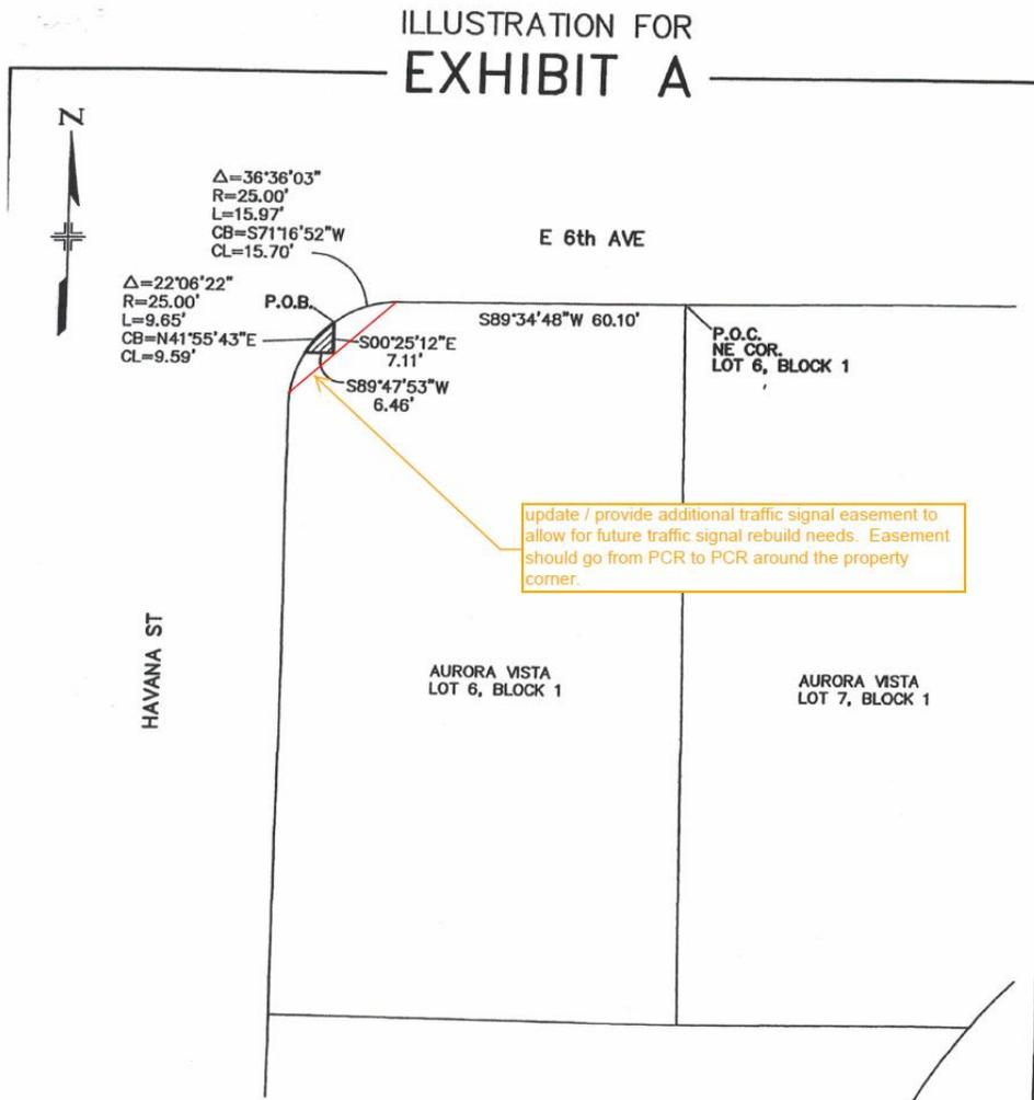
BEARINGS ARE BASED ON THE NORTH LINE OF LOT 6, BLOCK 1, AURORA VISTA, BEING  $S89^{\circ}34'48''W$ .
