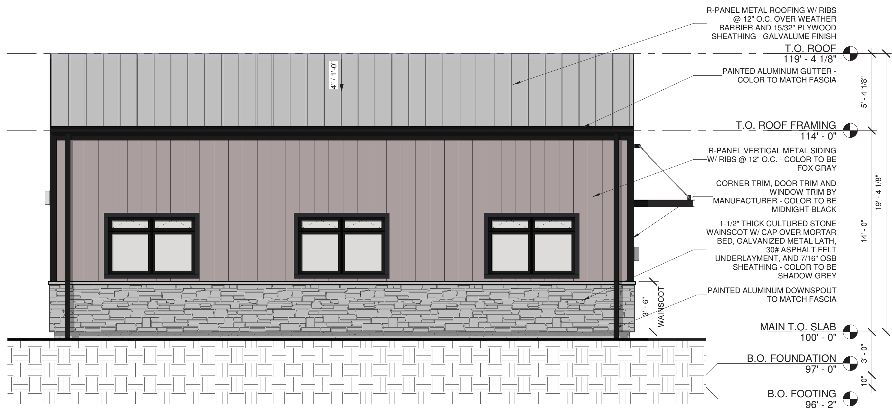
4 EAST ELEVATION - BUILDING 1 1/4" = 1'-0"
