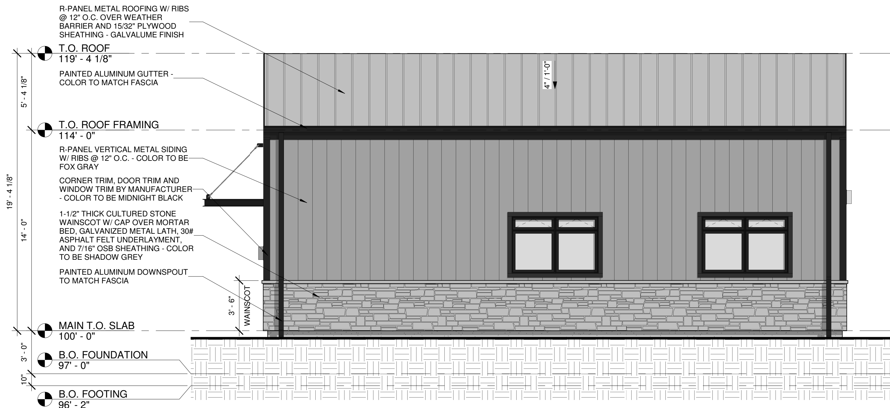
3 WEST ELEVATION - BUILDING 1 1/4" = 1'-0"
