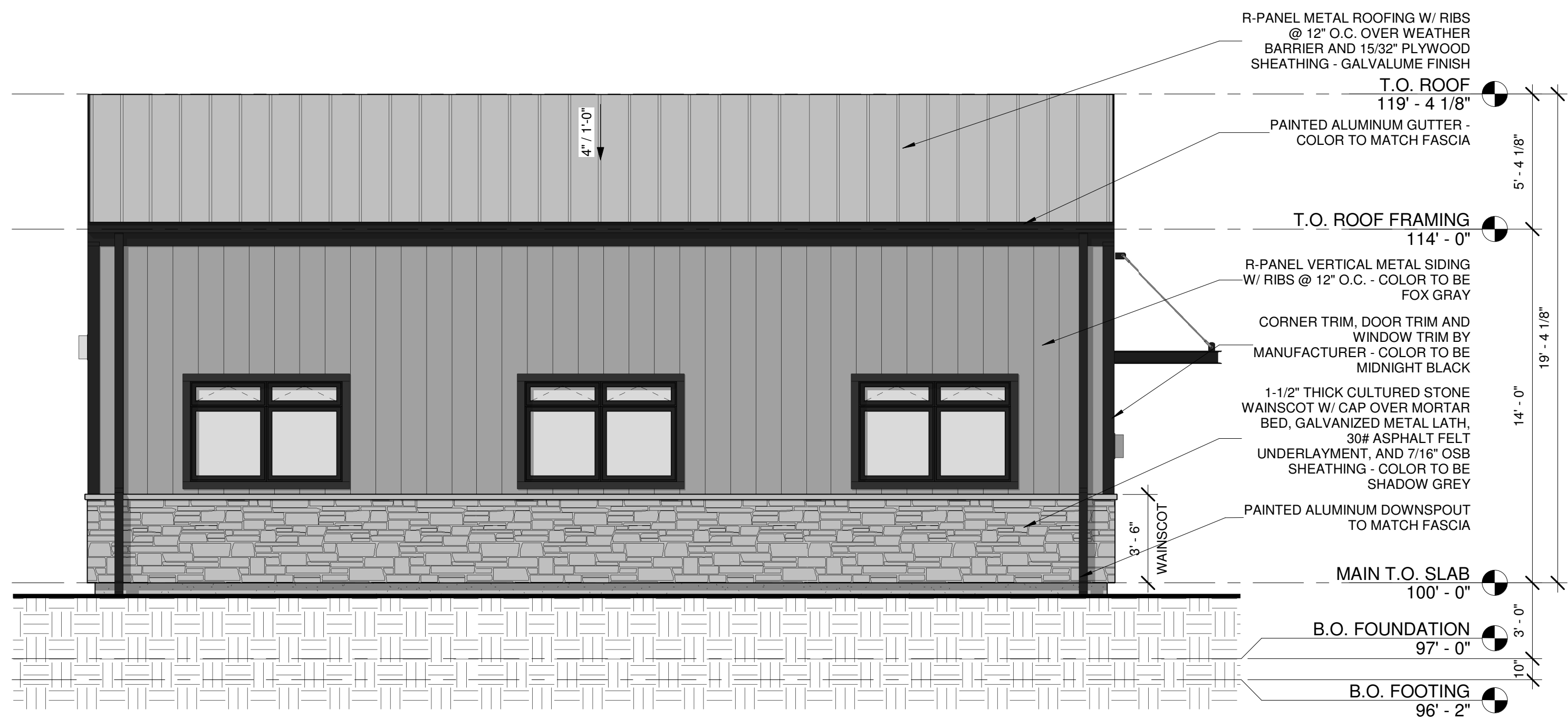
4 EAST ELEVATION - BUILDING 1 1/4" = 1'-0"
